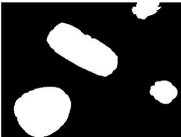
Fig. 4. Virtual object boundaries obtained after leaving some space around obstacles
